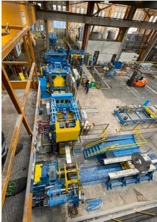
Civate plant - Roll levelling and cutting to length system with automated packaging
